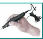
Figure 26. Hand engraving tool for metal identification tags.
