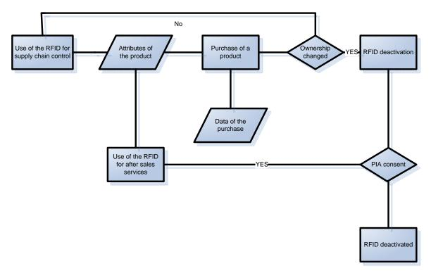
Figure 13. Flowchart of the process at the POS relevant for the RFID
