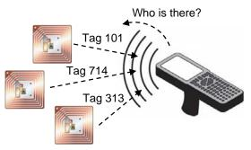
Figure 4. A tag singulation example
