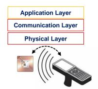
Figure 3. Tag-Reader communication architecture
