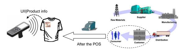
Figure 5. The reference scenario: supply chain and working RFID tags after the point of sale
