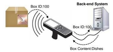
Figure 2. Typical scheme for RFID tags used for item labeling
